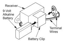
Figure 38 - Attaching Alkaline Battery to Receiver
